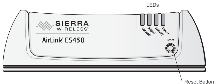
Figure 1-2: ES Series Device Front Panel
